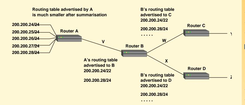
Routing **CIDR Aggregating Routes** Aggregating routes Without Route Summarisation With Route Summarisation Explanation How the Routes were Summarised Route Aggregation: NetAddr::IP route-aggregate Addressing Scheme BGP: AS Types **BGP Attributes** Preferring One Link **BGP Messages**
